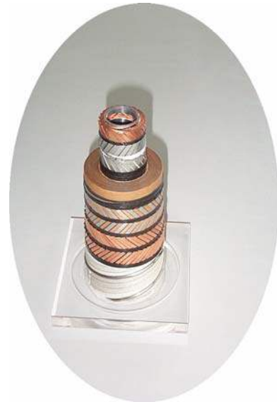
Photo 2 single phase CD cable (without cryostat)
