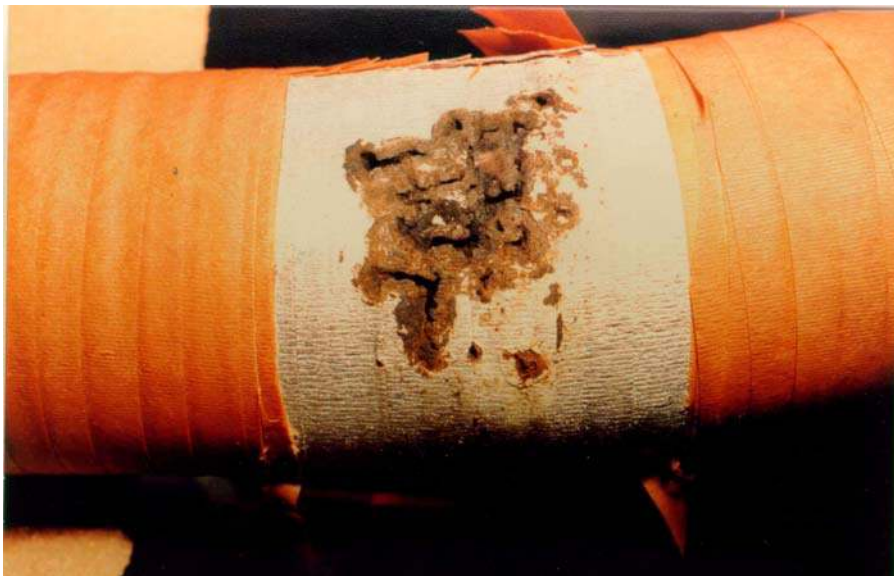
Mode 2: Dielectric overstressing and partial discharge activity
