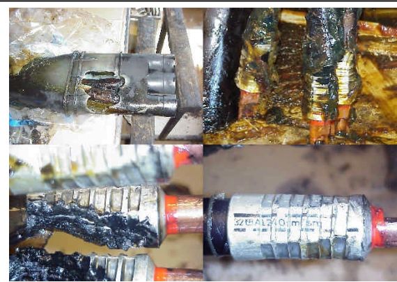
Figure 3.4 Fault cause analysis of disturbed cable termination. Several sharp edges on the connector were found on all three phases.
