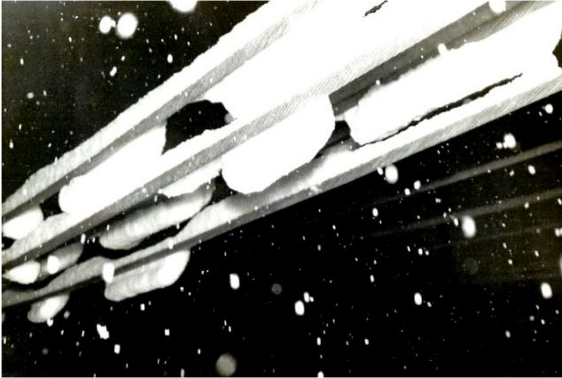
Figure 5: Dry snow accretion on overhead conductors
