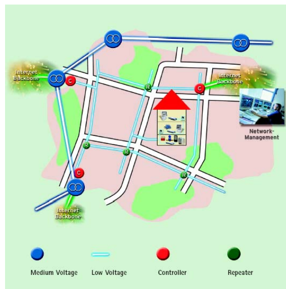
Figure 4-1 Typical PLC network architecture
