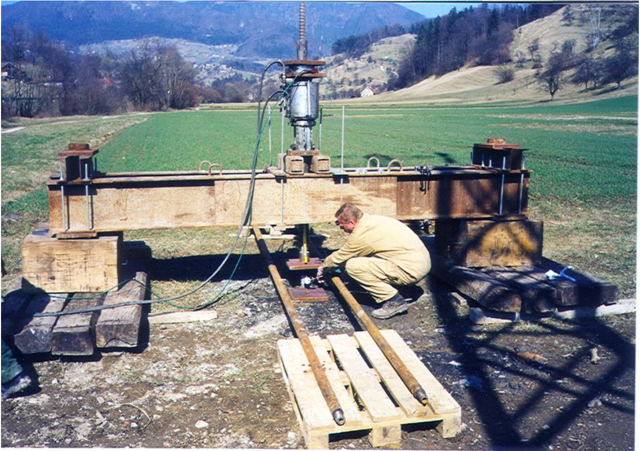
SLOVENIA, Micropile tensile strength test
