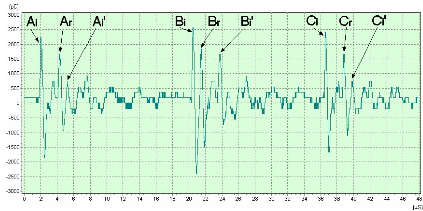
Fig. 19: Multiple PD events occurring during a time span of only 45\mu\text{s}
