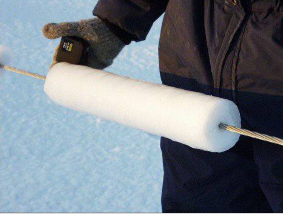
Figure 9 - Heavy radial ice buildup on a relatively small bare overhead conductor.
