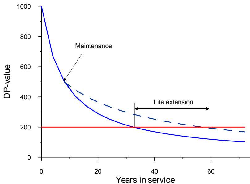
Figure 33: Simulation of maintenance action of cellulosic insulation and its effect on retarding ageing.
