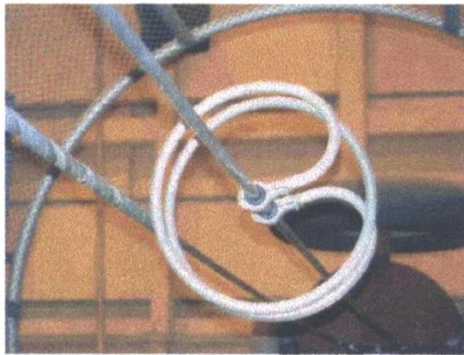
Figure 7.4: Hoop spacer used to maintain separation of sub conductors in despacered bundles [Hoffman & Tunstall, 2003]
