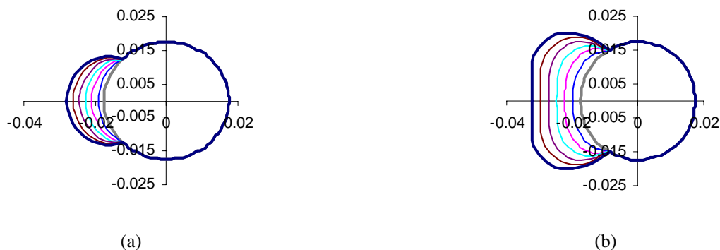
Figure 7.12: Comparison of ice shapes (based on [Lozowski et al, 1983]) (a) Case 1: air speed 5 m/s (b) Case 2: air speed 10 m/s
