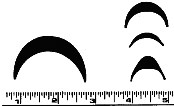
Figure 6.23: Plastic test foils used to simulate natural ice deposits [Nigol and Clarke, 1974].
