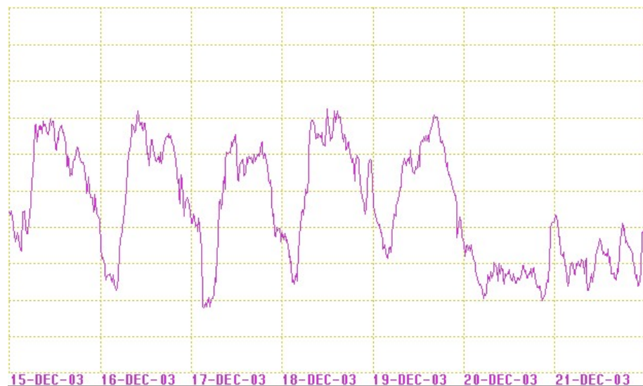
Figure 8: Typical daily load variation over one week for a 150 kV line
