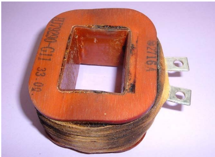
Fig. 3.2 Typical Coil Failure
