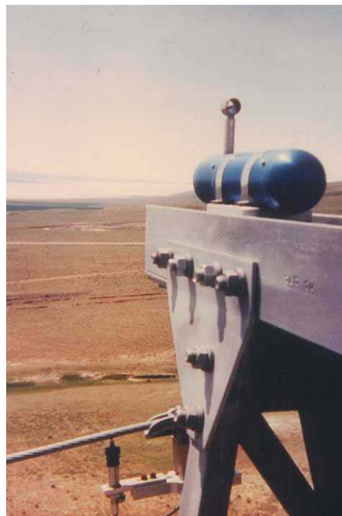
Figure 19: Vibration recorder Vibrec 400 with split displacement transducer.
