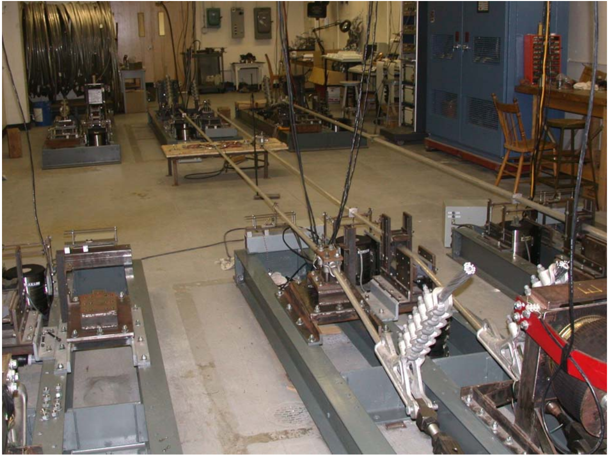
Figure 2b: Resonance type test benches, GREMCA's laboratories.
