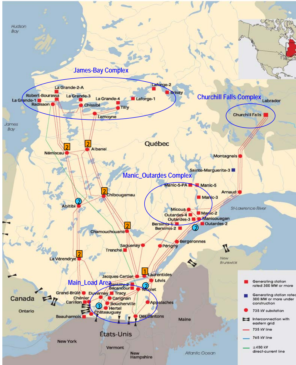
Figure 6.2.1. Dynamic shunt compensation units in Hydro-Quebec main grid: (2) Synchronous Condensers and (1) Static VAR Compensators.
