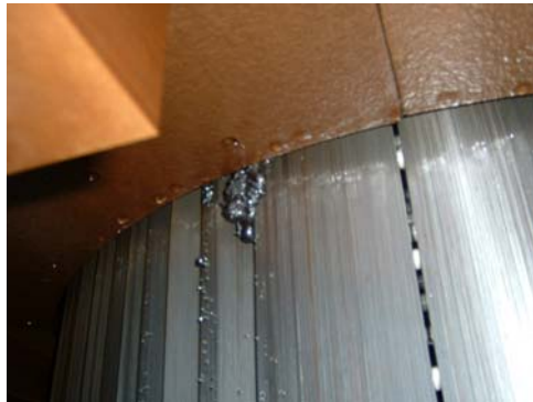
Figure 40: Shorted core laminations.
