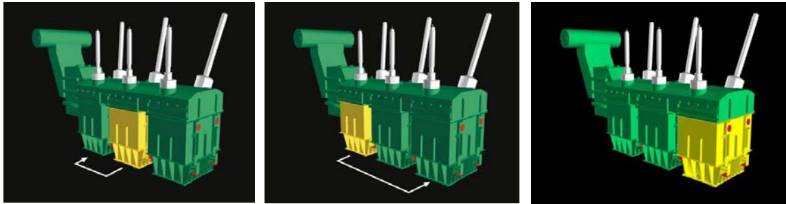
Figure B-8-1: On-site replacement of any phase
