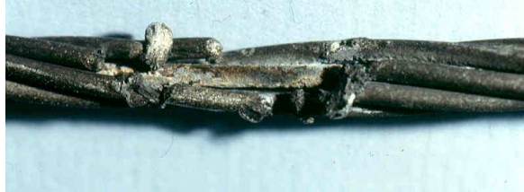
Figure 6-15: Clashing Conductors or Lightning Strokes may Lead to Electric Arc Burn
