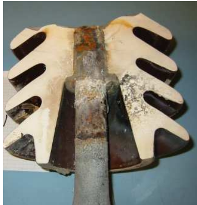
Figure 6-7: Corrosion on a Support Insulator
