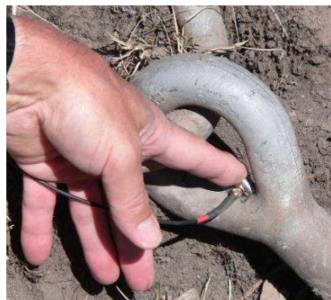
Ultrasonic NDE sensor placed in anchor rod eye
