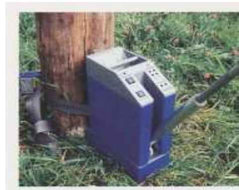
Control of embedding with the support of a dedicated tool: on this picture, the polux device, used to analyse the residual wood properties
