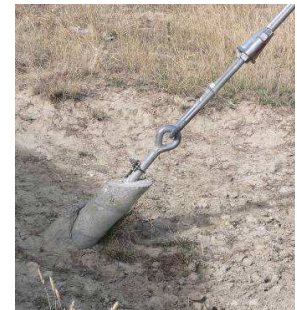
Anchor rod with grout exposed from erosion
