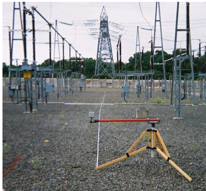
Figure 9 : insulating tripod and offset rod for an electric field probe (photograph RTE)
