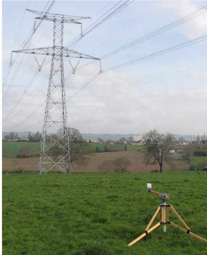
Figure 5 : electric field probe and insulating support (photograph RTE)
