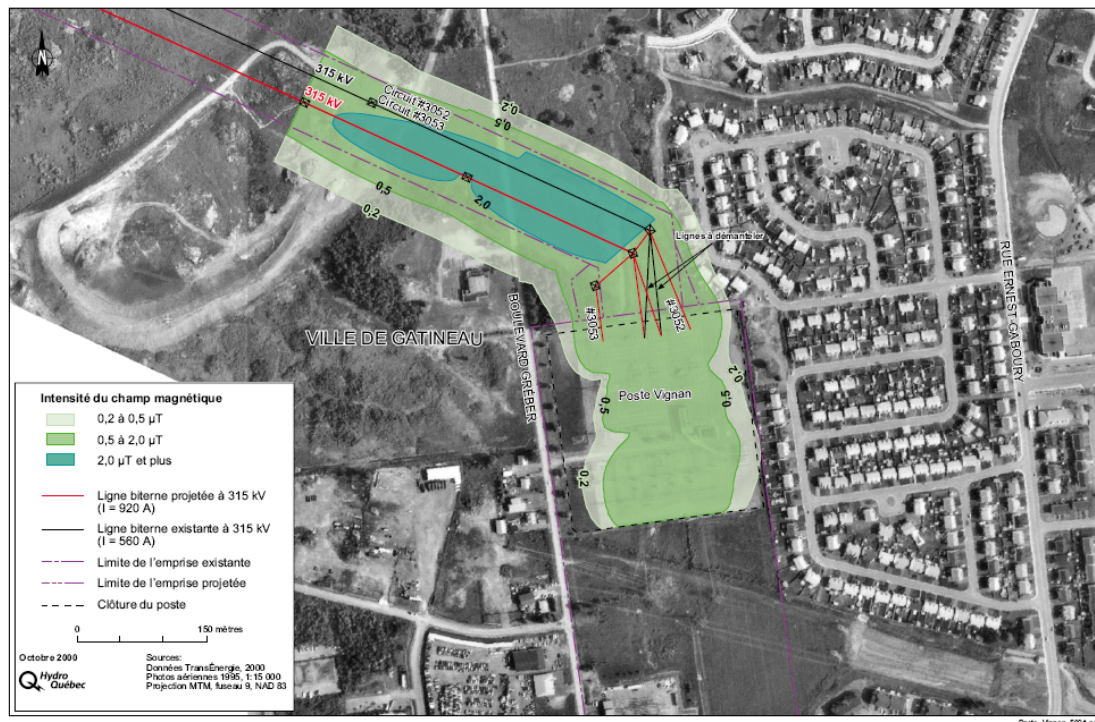
Figure 18 Electric and magnetic field (EMF) representation. (Source : Hydro-Québec, 2007)
