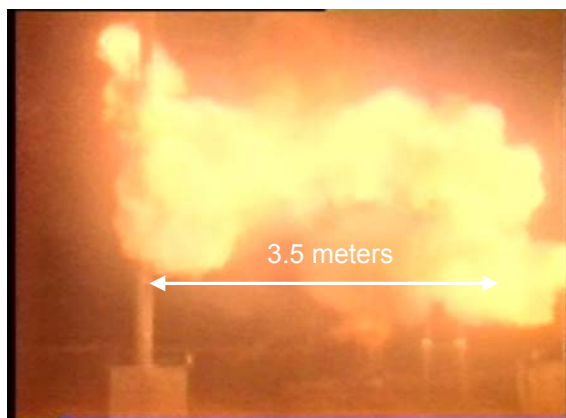
Figure 9: Appearance of a 30 kA power arc
