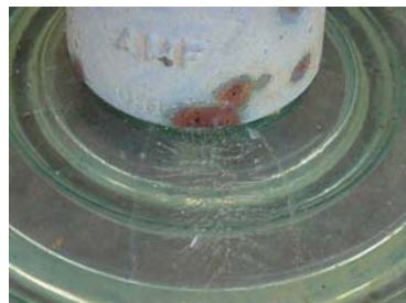
Figure 5.4: Damage on a glass disc /9/
