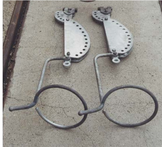
Figure 8.2: End fitting after short circuit testing
