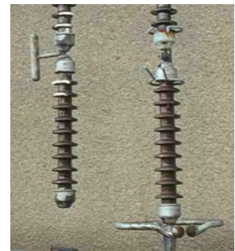
Figure 5.3: Results of different arc protection
