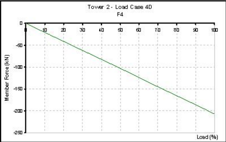
Figure 21: Results of calculation of member F4, for prototype 2, and LC 4D
