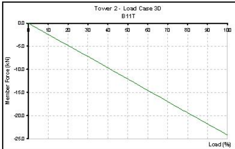
Figure 28: Results of calculation of member B11T, for prototype 2A, and LC 3D
