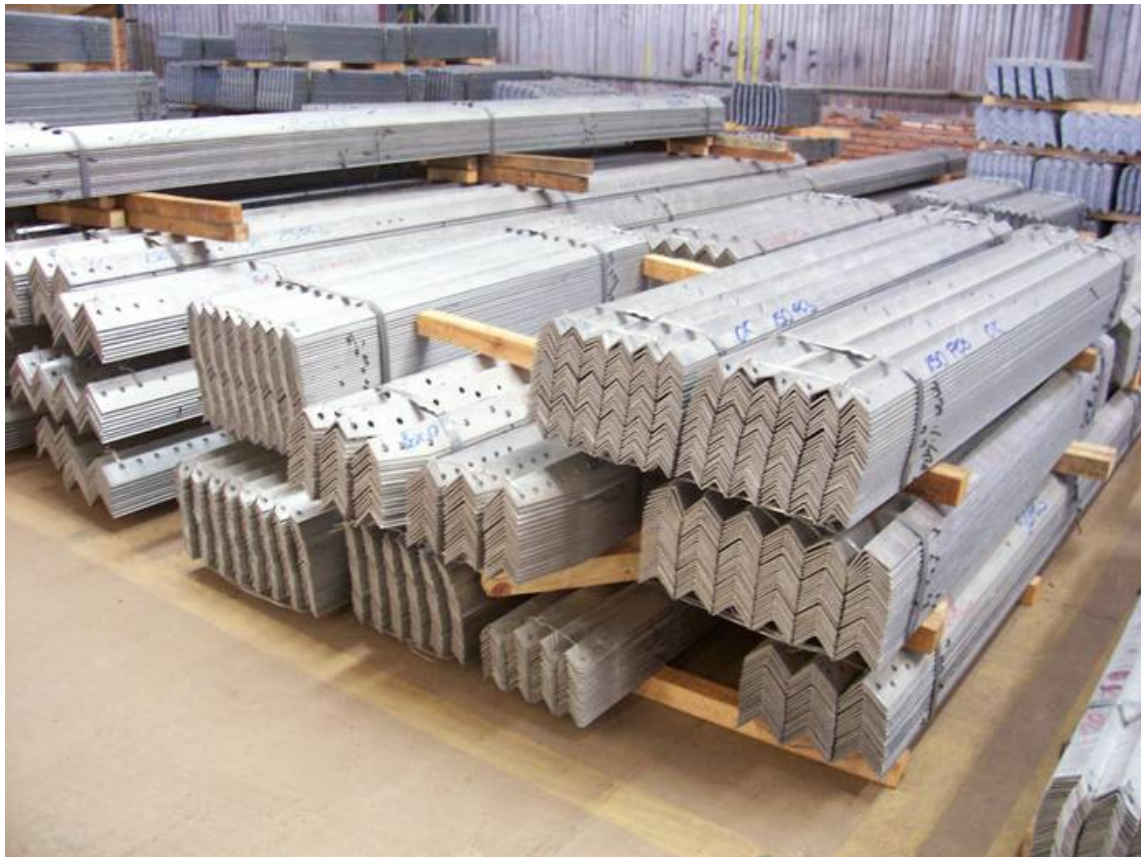
Figure 4 – Galvanized lattice steel members
