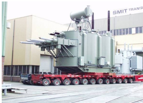
Figure 2 - 400 kV 1 phase unit (dimension 8x6x6 m weight: 550 ton)
