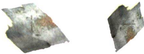
Fig 1g Copper sulphide formation on heavily aged papers from a failed industrial transformer.
