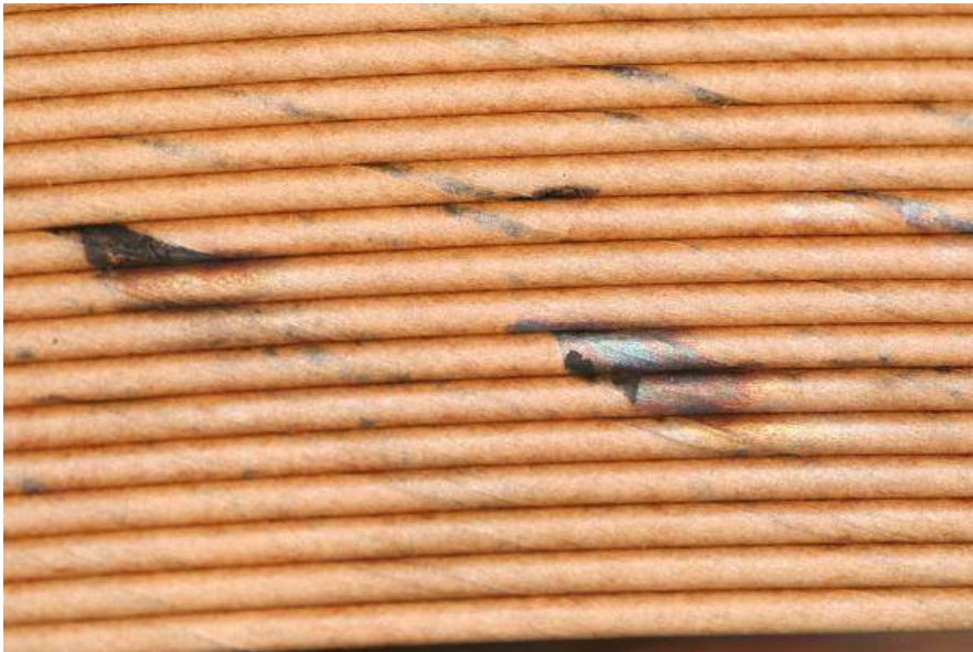
Fig. 3. Initial stage of failure. Copper sulphide has grown through all layers of paper, showing as a metallic layer on the surface. There are traces of discharges between conductors. From a disc of a valve winding (neighbouring phase to failed one) in a HVDC transformer.
