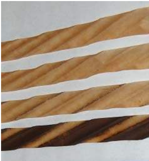
Fig. 1b Contaminated covering paper, note the dark colour easily mistaken for sludge, from [24]
