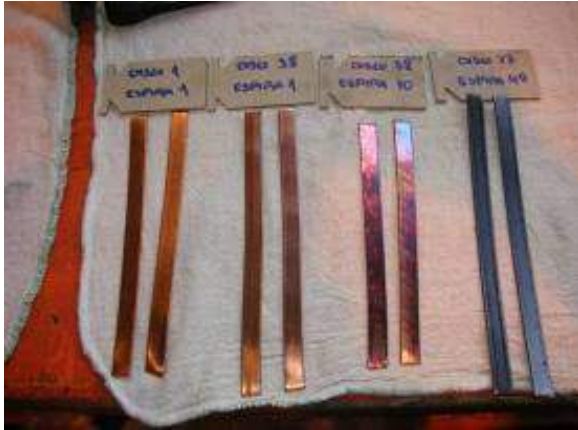
Fig 1a Discolouration of copper conductors from a failed shunt reactor, from [24]
