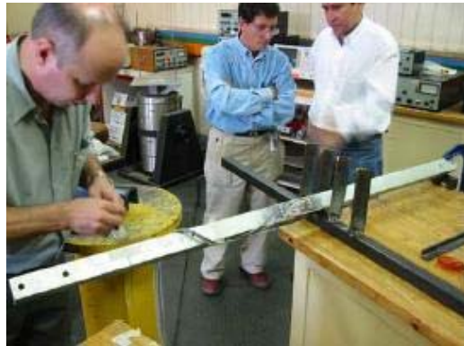
Figure 8: Calibration of a strain gaged member
