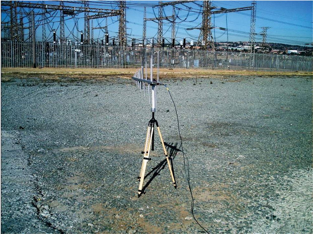
Figure 7: RFI measurement in the frequency range 30 MHz to 1 GHz.
