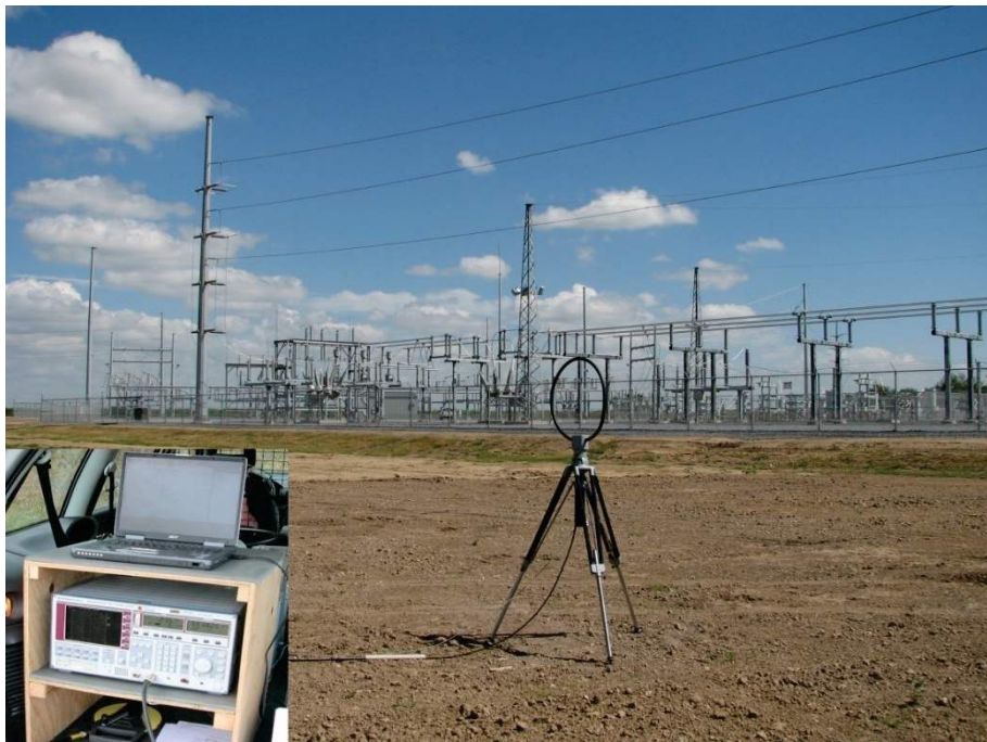
Figure 1: RFI measurement in the frequency range 9 kHz to 30 MHz.
