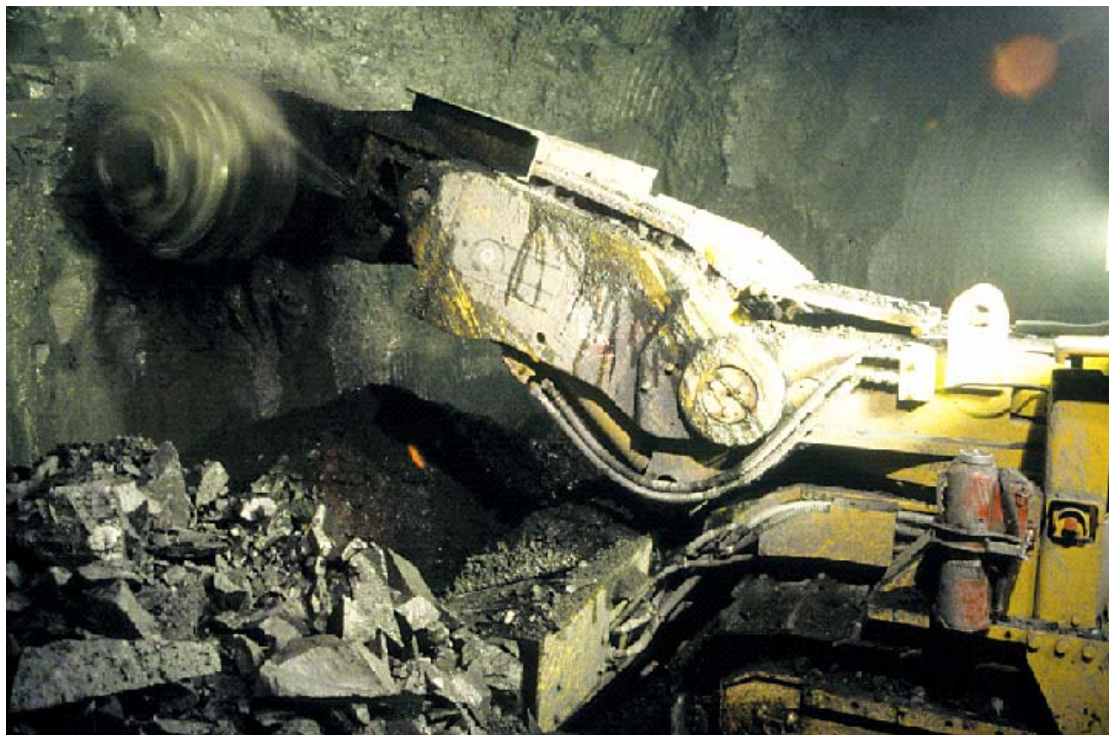
Fig. 2.1.9 A road header machine with boom mounted cutter head.
