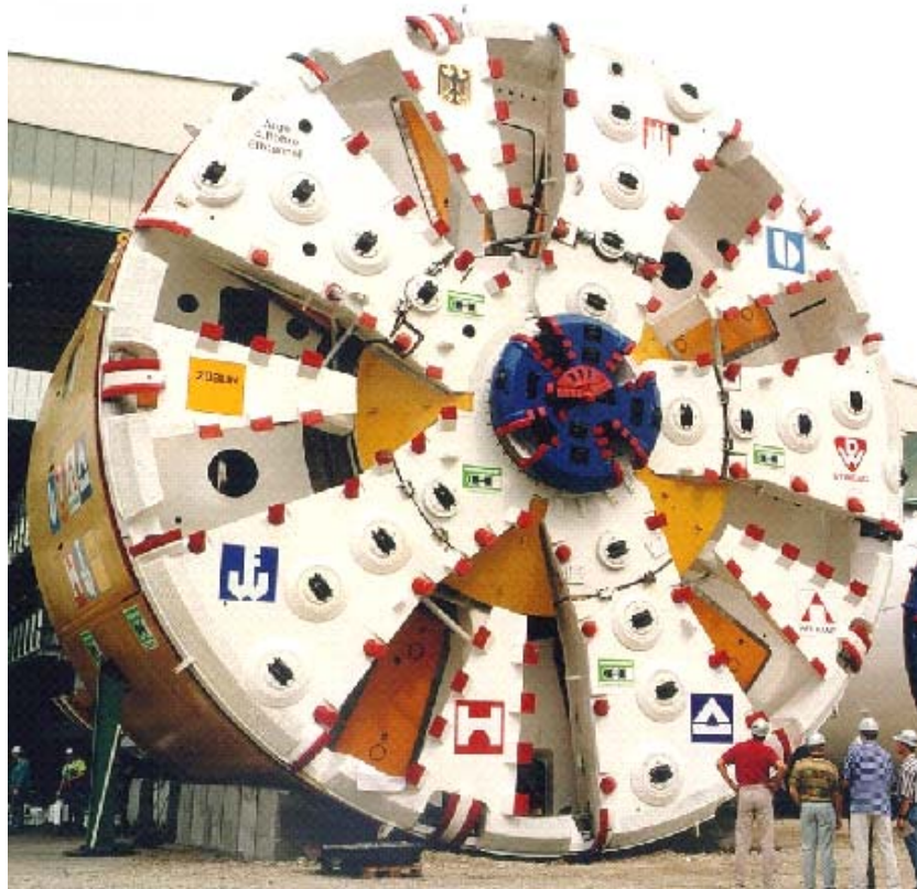
Figure. 2.1.4 The cutting head of a large diameter Tunnel Boring Machine (TBM)
