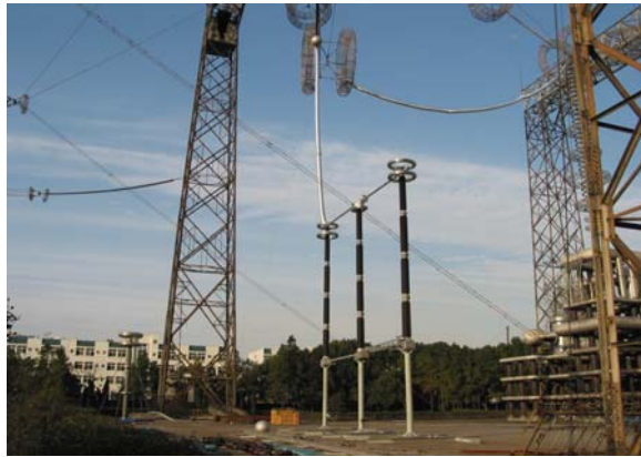
Fig. 24 Electromagnetic field test set-up for UHV disconnector
