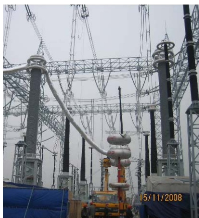
Fig. 111 On-site HV test set-up (left) and typical test procedure (right)
