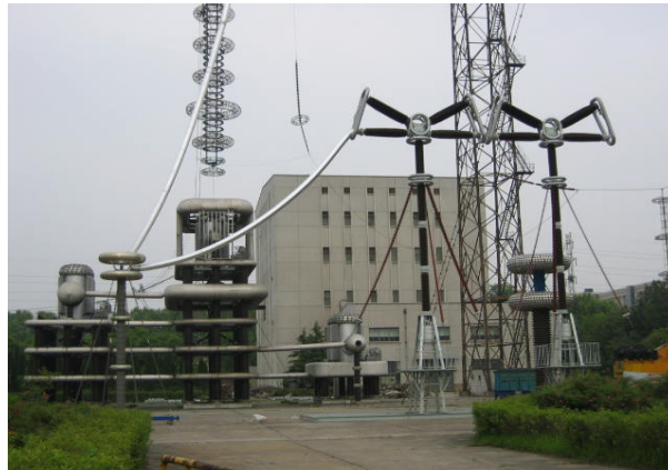
Fig. 21 Electromagnetic field test set-up for UHV SF 6 circuit breaker
