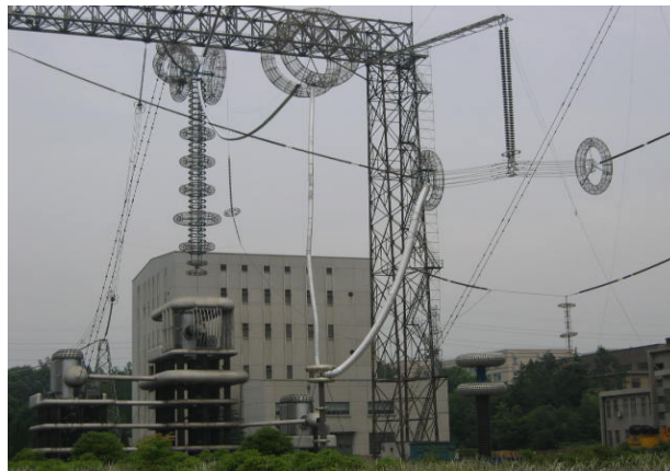
Fig. 22 Electromagnetic field test set-up for UHV double suspension insulator strings
