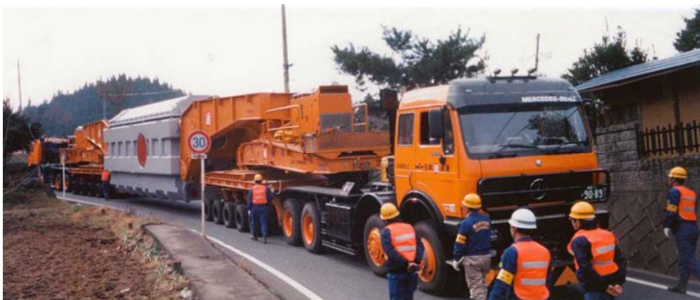
Fig. 18 Transportation of UHV transformer to the site in Japan
