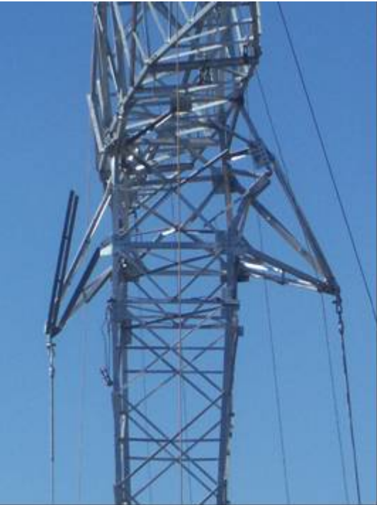
Figure 17 – Guy cross arm fail by tension Failure when completing 120% on a destructive test
