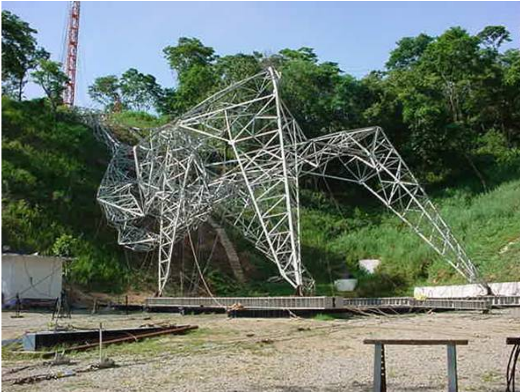
Figure 9 – Destructive test - 500 kV TL Tower
