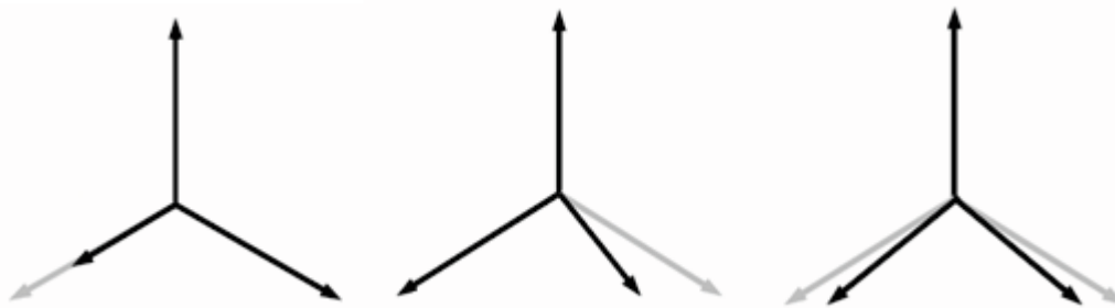
Figure 6-1 Testing vectors 3A, 3B and 3C according to IEC 61000-4-34.
