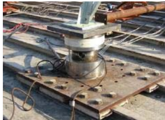
Figure 7: Device designed for foundation displacements
