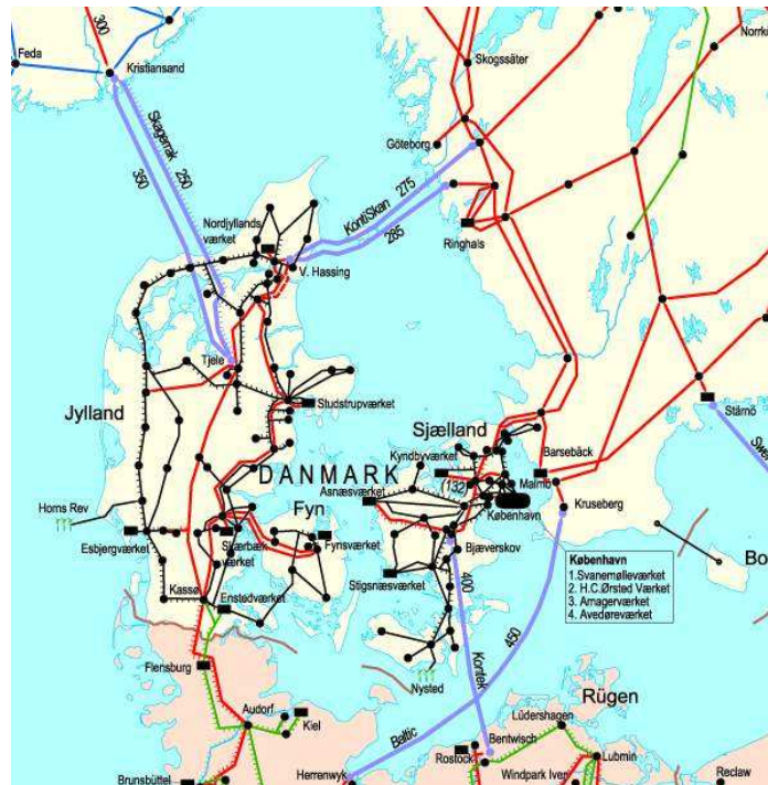
Figure 26: The Danish power grid 132-400 kV including HVDC links to neighbouring countries. This grid consist of approx. 1000 km of 400 kV overhead lines, 70 km of 400 kV PEX Cables, 500 km HVDC cables/overhead lines and approximately 3000 km of 132-150 kV overhead lines.
