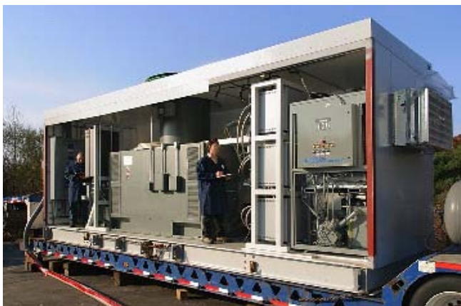
Fig. 3.9: 8 MVAR dynamic synchronous condenser for TVA test site
