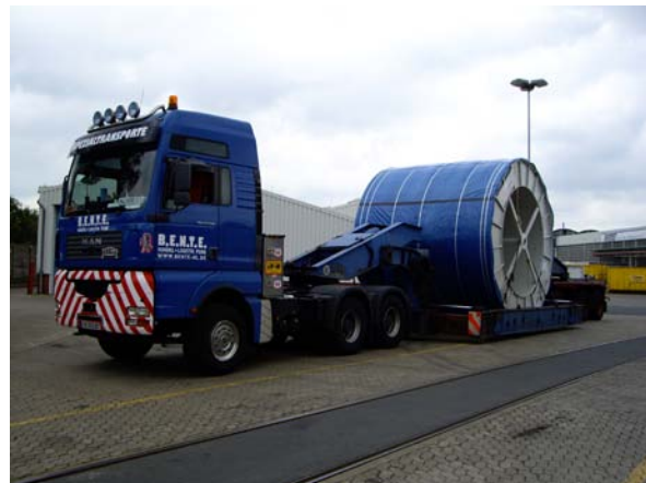
Fig. 4.6: 600 m HTS cable with evacuated cryogenic envelope on one drum
