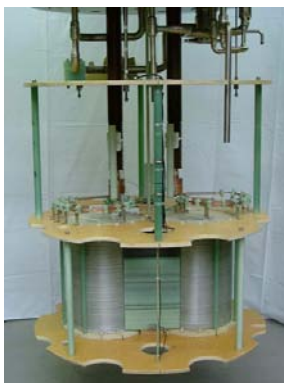
Fig. 6.2: SMES coils for 25 MW pulsed power modulator
