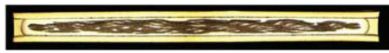
Fig. 2.1: Cross-section of 1 G HTS wire, showing 55 filaments (black) embedded in silver, laminated on both sides by stainless steel. (Courtesy of American Superconductor)
