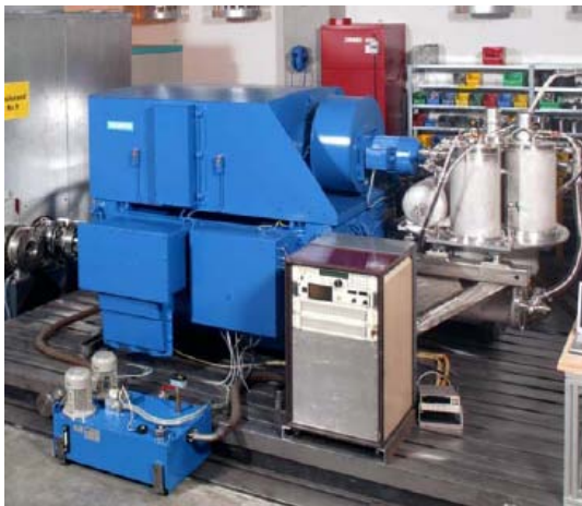
Fig. 3.6: 4 MVA HTS machine
