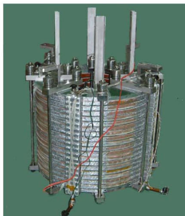
Fig. 6.10: A 1MJ-class SMES coil for bridging instantaneous voltage dips.
