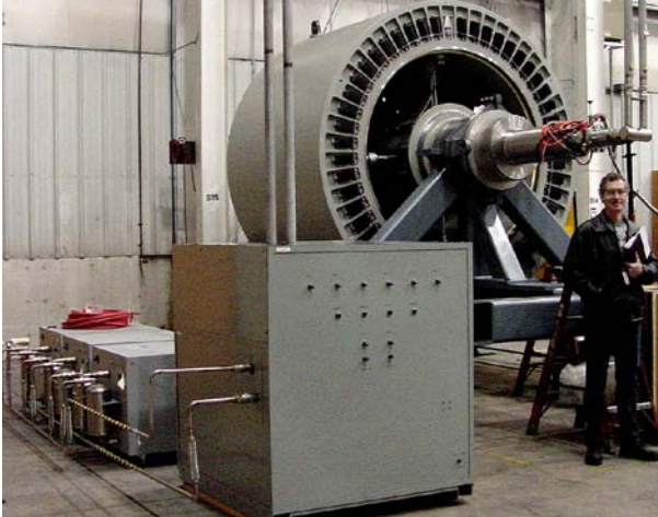
Fig. 3.5: Rotor and rotor cooling system during factory testing prior to shipment to Philadelphia
