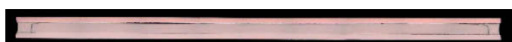
Fig. 2.4: Cross-section of a 4.4 mm wide laminated wire, called 344 superconductors by American Superconductor, showing three layers: two copper laminates on the top and bottom, and a central insert consisting of a NiW substrate coated with here-invisible buffer and HTS layers. (Courtesy of American Superconductor)
