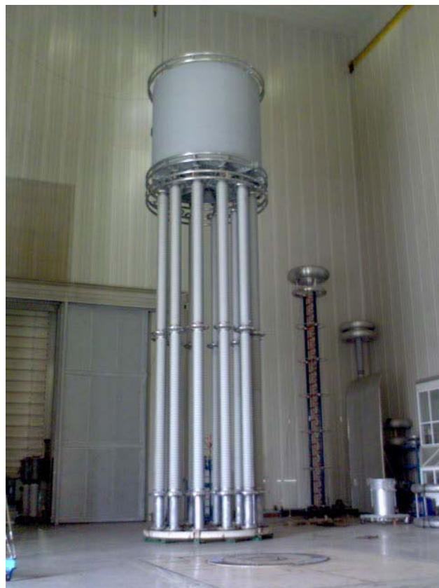
Figure 3.9- Air Core Smoothing Reactor under testing (Courtesy Siemens)
