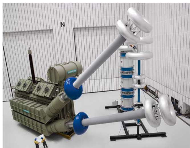
Figure 3.4 – 800 kV Converter Transformer under testing (Courtesy Siemens)
