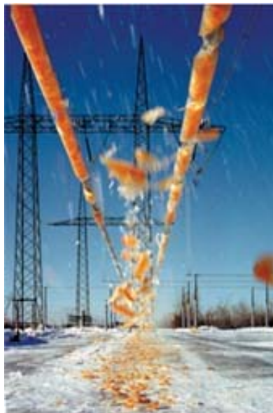
Figure 7.8: EIDI of twin bundle using 10 kA and appropriate reclosing sequence [91]
