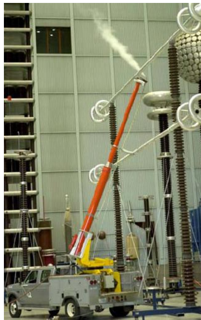
Figure 7.17 : Remote steam de-icing vehicle [115]
