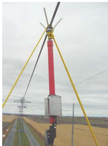
Figure 7.7. DAC prototype held in place by a taut rope and ready to be fired [89]
