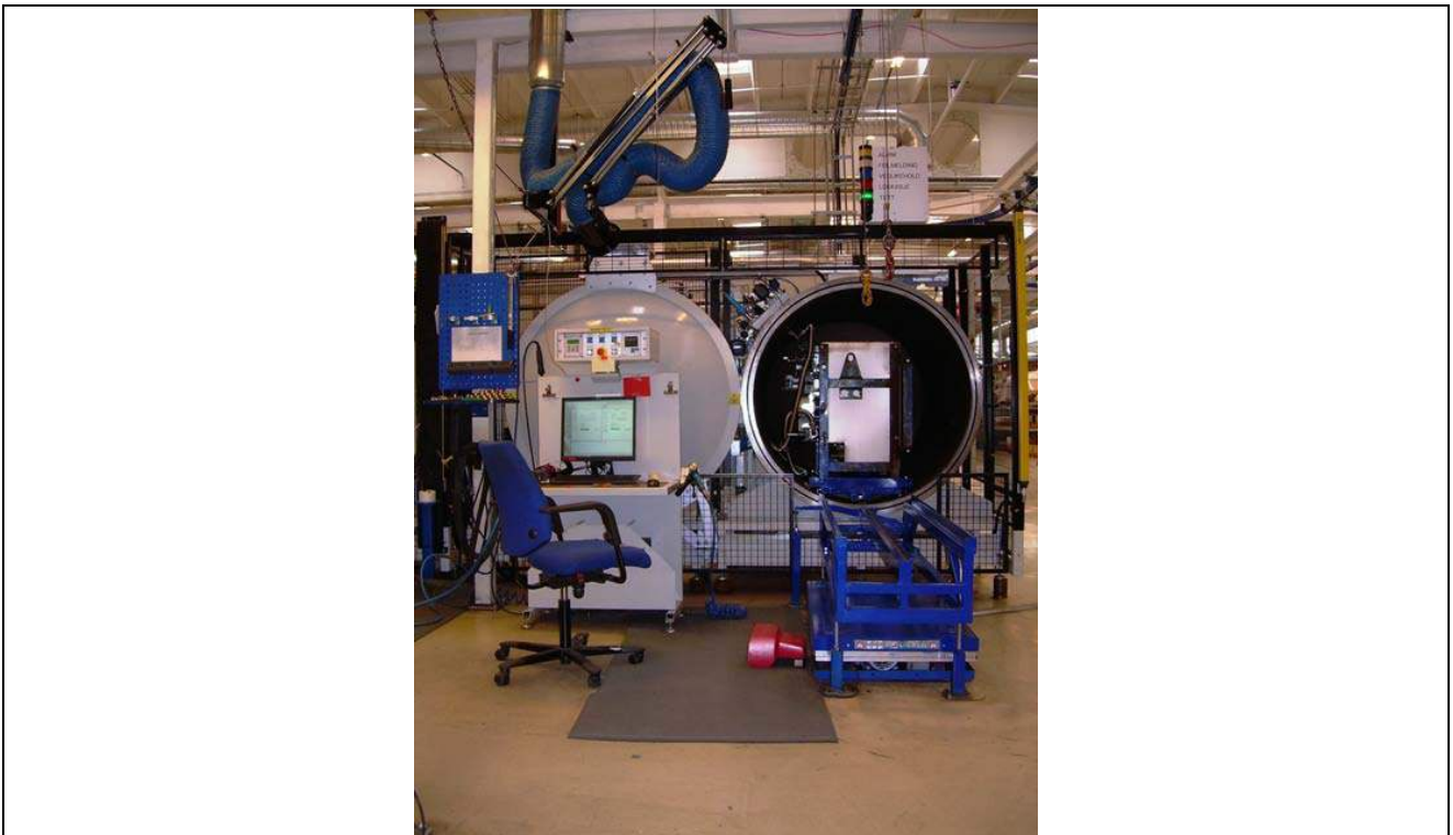
Figure 5: Helium leakage test device used for routine testing of Ring Main Units. The RMU is visible inside the chamber.
