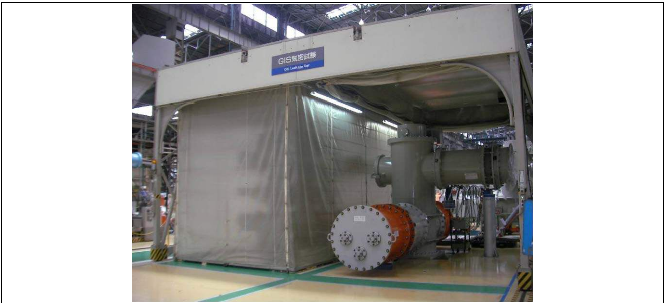
Figure 14: Leakage test with defined accumulation volume (example with Gas Insulated Switchgear)
