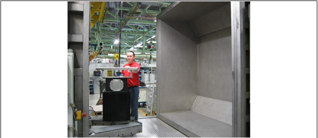
Figure 4: Helium leakage test chamber used for routine testing of large medium-voltage equipment. A complete functional unit of a switchgear can be placed between the two halves.
