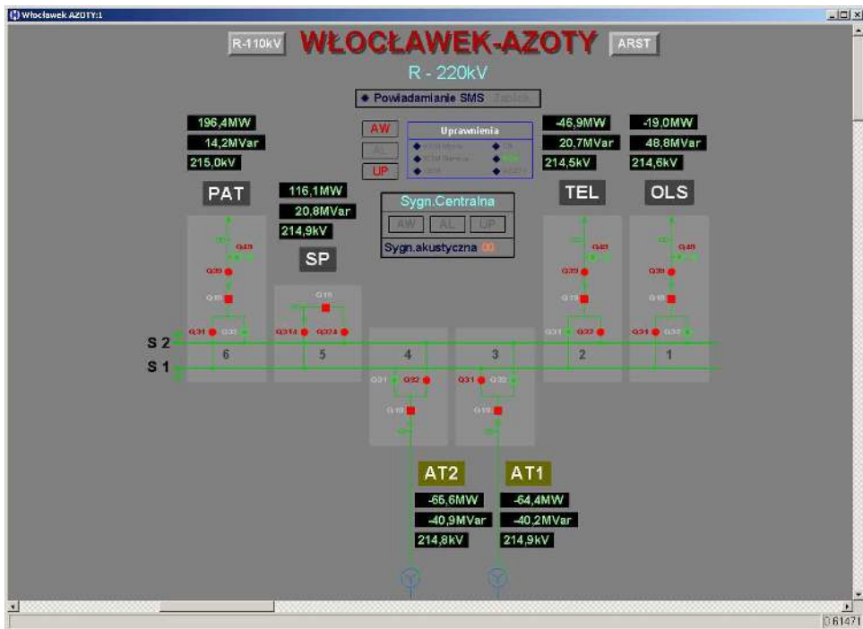
Figure 8: Substation layout on the local HMI
