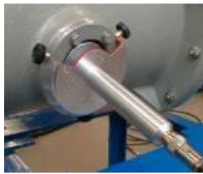
Fig. 2.4: Sectional view and mounting of an UHF PD mobile window coupler
