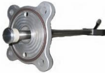
Fig. 3.3: UHF probe, mounted on the oil filling valve (DN 80) pushed inside the transformer [14]
