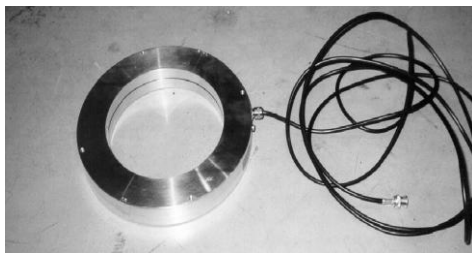
Fig. 2.2: a) Examples of different PD sensors b) Rogowski coil, bandwidth 5 MHz – 100 MHz
