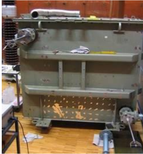
Fig. 5.18: Test tank with two oil valves and two flange-mounted UHF probes
