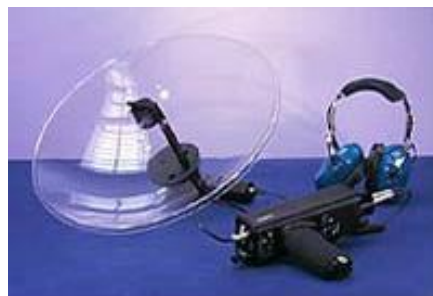
Fig. 3.19: Ultrasonic measuring instrument with directional microphone:
