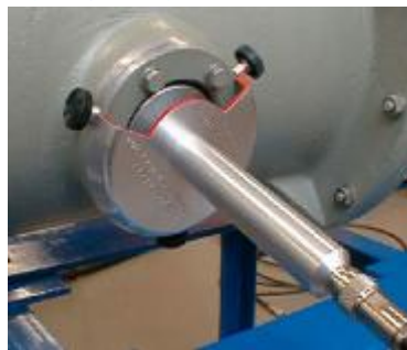
Fig. 3.7: Sectional view and mounting of an UHF PD mobile window coupler [1, 28]
