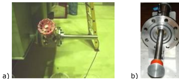
Fig. 2.6: a) UHF oil-valve sensor applied to a power transformer b) Disc-shaped UHF sensor for a standardized oil-valve for online applications
