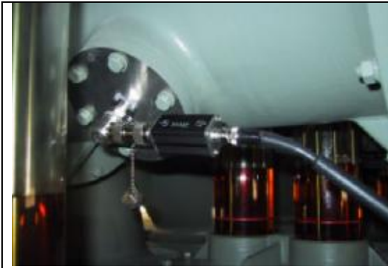
Fig. 3.9: External window sensor with preamplifier [15]
