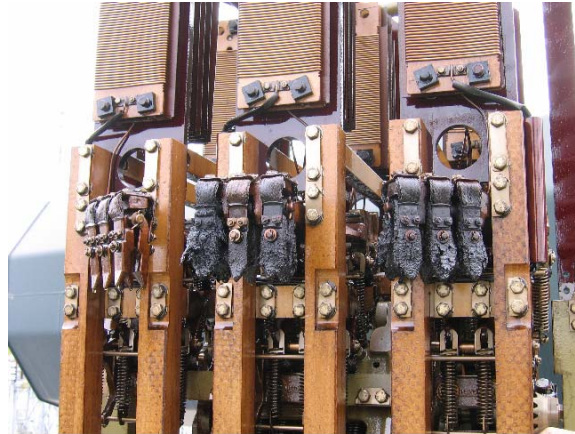
Figure 1: Example of heavy coking on LTC contacts 28
