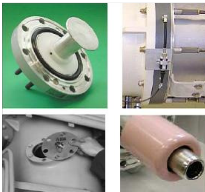
Figure 8.2.1 Different types of PD couplers for GIS [5]
