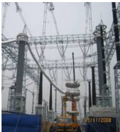
Figure 8.2.3 On-site HV test set-up (left) and typical test procedure (right)
