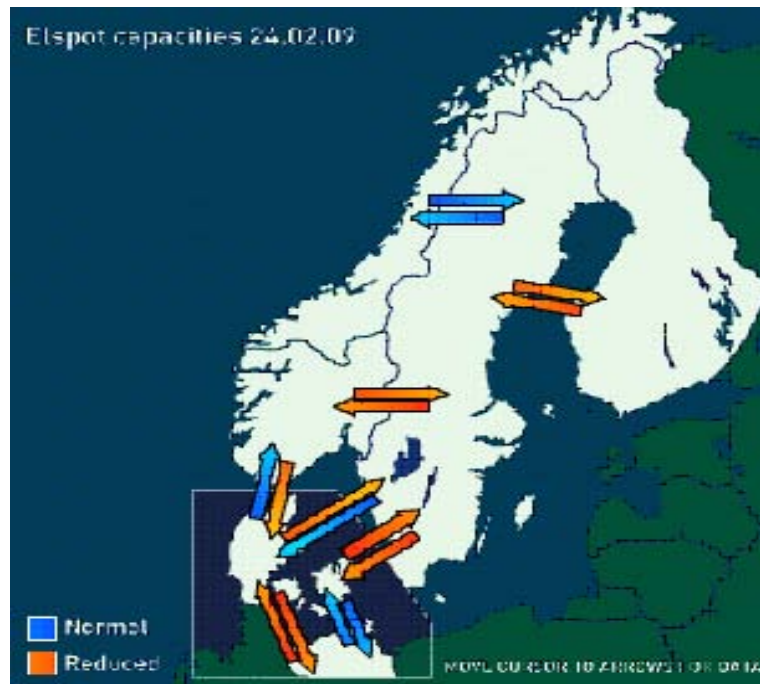
Figure 2-8 The actual situation of the critical exchange points. Blue indicates normal operating conditions; orange indicates reduced transfer capacity [25]
