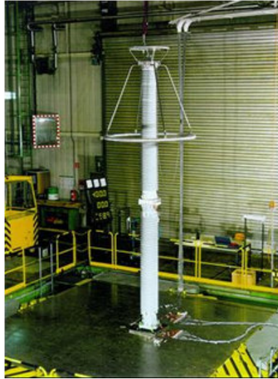
Figure A-7.1.3: Seismic test on a polymer housed surge arrester (composite hollow core insulator) for a 550 kV system.
