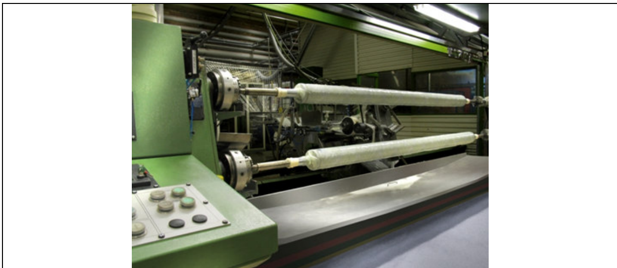
Figure 2-11: Wet winding of tubes for composite insulators
