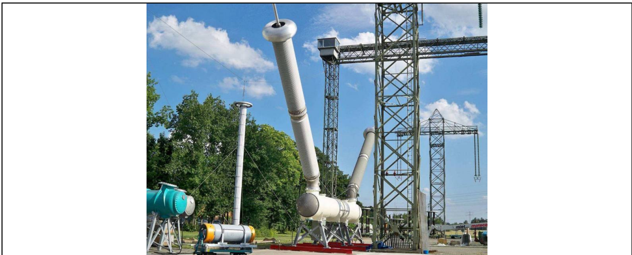
Figure 11-6: Fig, 6 1100 kV circuit-breaker with composite bushings [11.15]
