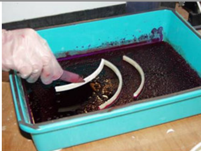
Figure 4-3: Example of design test. Tests on the tube material. Dye penetration test (Note – the length of the test sample presented in this figure is much larger than required by the standard)
