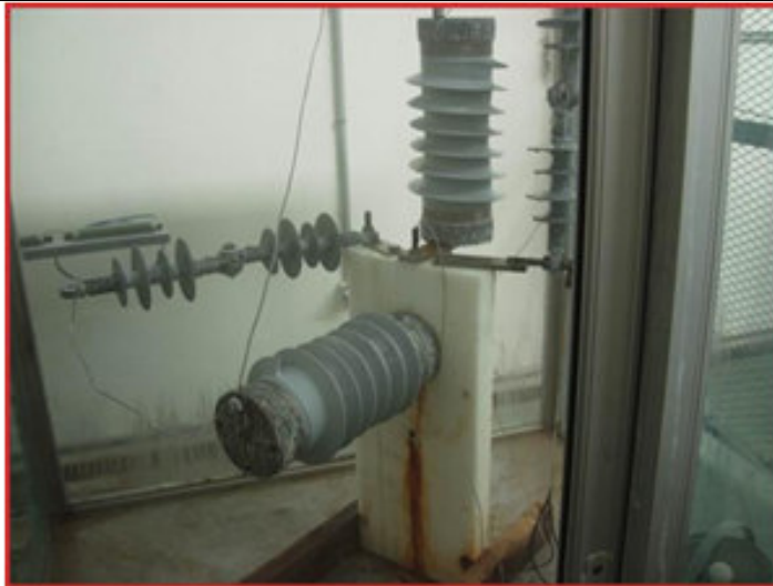
Figure 4-2: Example of design test. Tests on shed and housing material, item 7.3 of the Standard Tracking and erosion test (1000 hours salt fog test)
