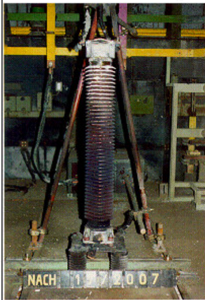
Figure A-8: Two porcelain housed arresters after high-current short-circuit tests [A-7.2.4]
