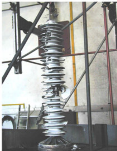
Figure A-10: Arrester with polymeric housing without internal gas volume after a high-current short-circuit test
