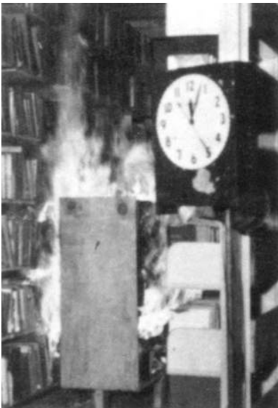
FIGURE L.1(f) Three Minutes, 25 Seconds; Active Burning in First Tier; Sprinklers Not Yet Operating.
