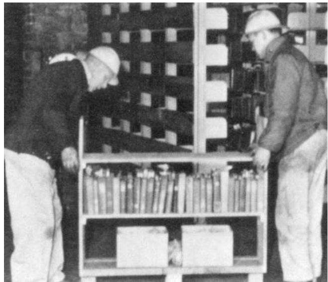
FIGURE L.1(d) Wood Book Cart Before Being Placed in Aisle of First Tier. (After placement, books were put on top shelf of book cart. The fire was started with an ordinary match by igniting the crumpled piece of paper between the two cartons on the bottom shelf of the cart.)
