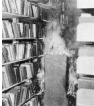
FIGURE L.1(k) After Approximately 3 Minutes; Active Burning in First Tier; No Sprinklers.
