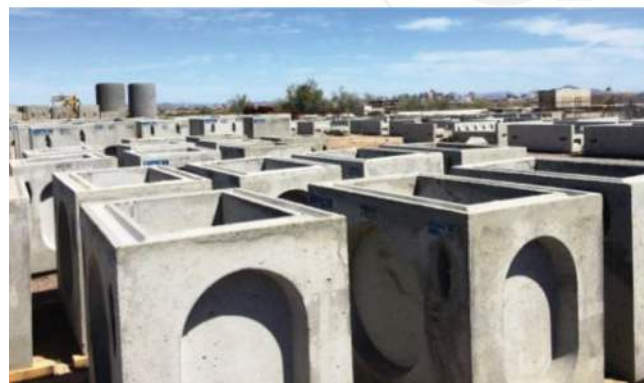
Fig. 5.5c—Synthetic macrofibers used in precast wave breakers and septic tanks.
