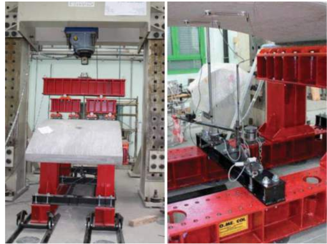
Fig. 5.5d—Flexural testing of segmental units reinforced with steel fibers (Moccichino et al. 2006).
